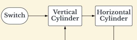
Operator pushes the switch, vertical cylinder moves down, O Vertical cylinder has lower initiating the horizontal cylinder cleans the chips and retracts back, finally the vertical cylinder goes back to home position
