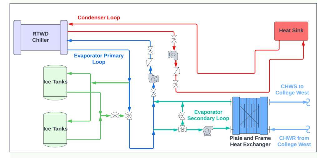
The primary mechanical components of the TES system includes a chiller, modular storage tanks, heat exchanger, pumps, piping, and valving.
