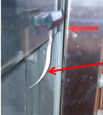
Paper fluttering into the fume hood
