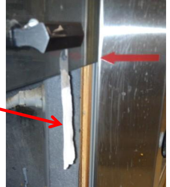
Paper not moving = no air flow
