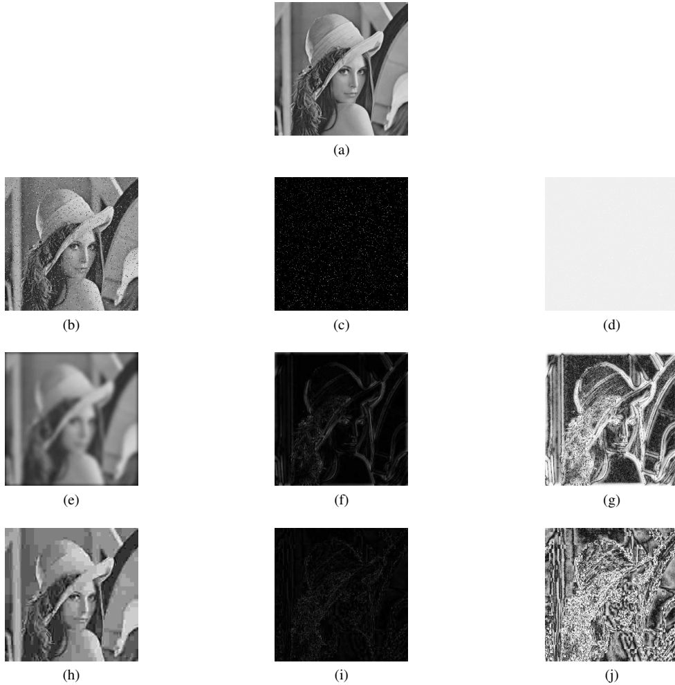
Fig. 2. MSE error map. (a) Original “Lena” image; (b) 6.25% random noise; (c) MSE random noise error map; (d) Equalized MSE random noise error map; (e) 15 \times 15 Gaussian blur; (f) MSE Gaussian blur error map; (g) Equalized MSE Gaussian blur error map; (h) 85% JPEG compression; (i) MSE JPEG compression error map; (j) Equalized MSE JPEG compression error map.
