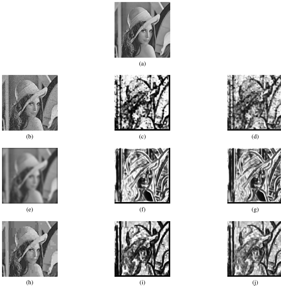
Fig. 5. SSIM error map. (a) Original “Lena” image; (b) 6.25% random noise; (c) SSIM random noise error map; (d) Equalized SSIM random noise error map; (e) 15 \times 15 Gaussian blur; (f) SSIM Gaussian blur error map; (g) Equalized SSIM Gaussian blur error map; (h) 85% JPEG compression; (i) SSIM JPEG compression error map; (j) Equalized SSIM JPEG compression error map.
