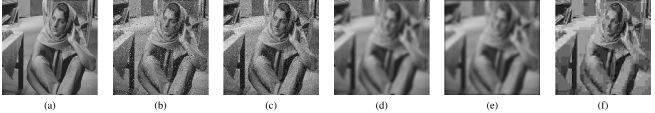
Fig. 3. Equal SSIM Hypersphere. (a) Original “Barbara” image; (b) 7.15% random noise, SSIM = 0.5033, MSE = 550.1926; (c) 14.5\sigma Gaussian noise, SSIM = 0.5036, MSE = 418.5383; (d) 9 \times 9 averaging blur, SSIM = 0.4989, MSE = 279.0549; (e) 13 \times 13 Gaussian blur, SSIM = 0.4767, MSE = 369.0773; (f) 90% JPEG compression, SSIM = 0.5028, MSE = 250.0337.
