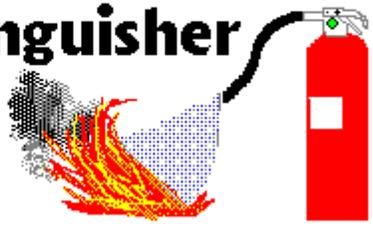
It's easy to remember how to use a fire extinguisher if you can remember the acronym **PASS**, which stands for **Pull**, **Aim**, **Squeeze**, and **Sweep**.
